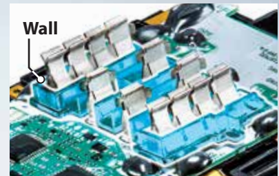
Terminal short-circuit prevention structure
